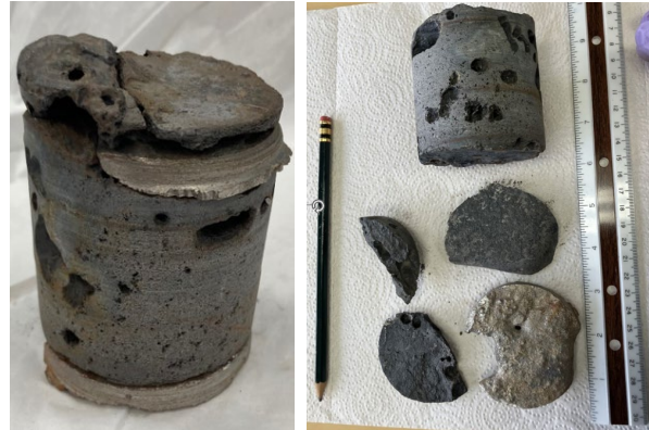
Figure 1. Core sample removed from reactor after MRE testing complete.
